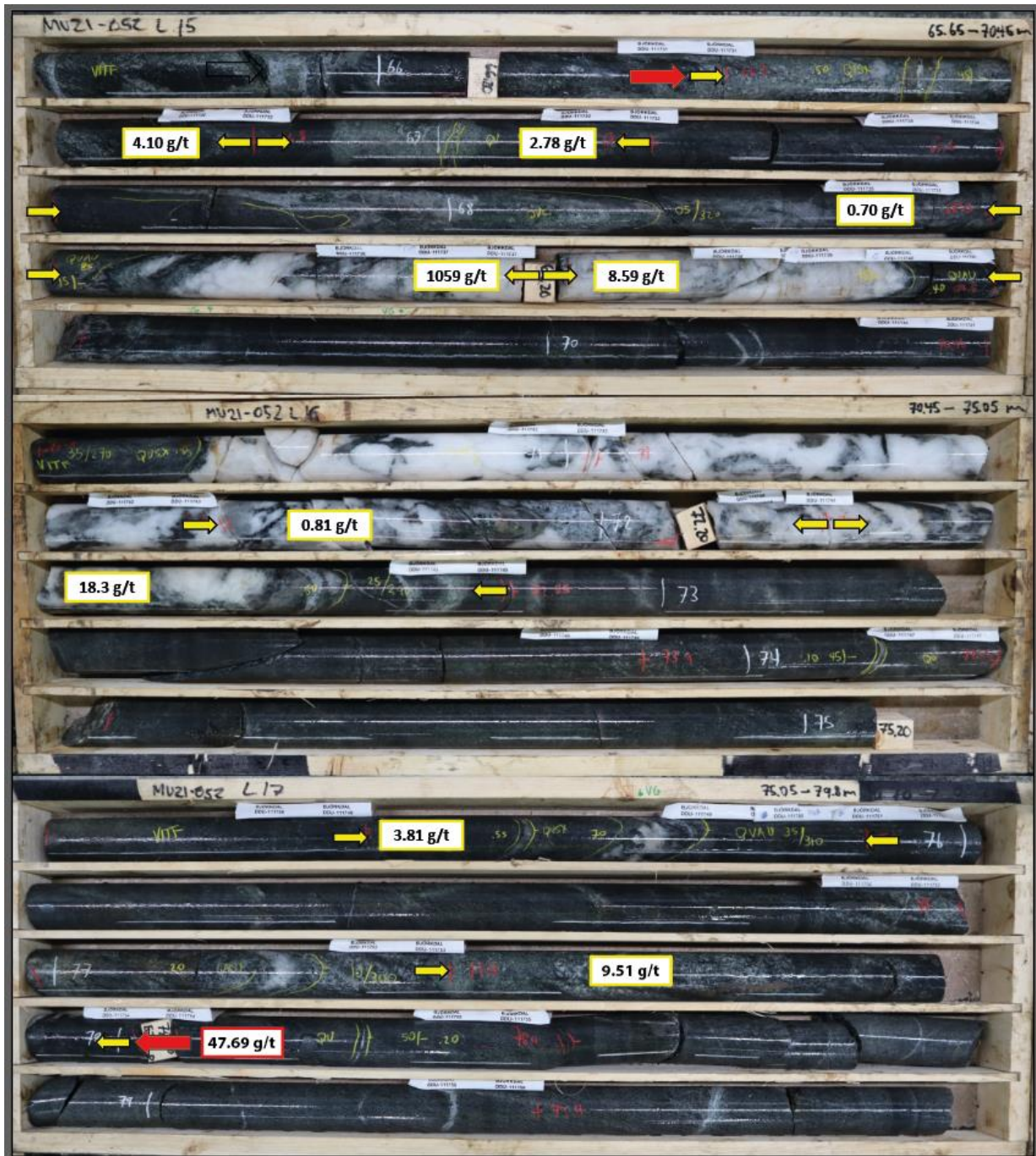
Figure 6. Photograph of a significant intercept within MU21-052 (66.3.7 – 78.0 m – ETW 5.85m @ 47.7 g/t Au).
