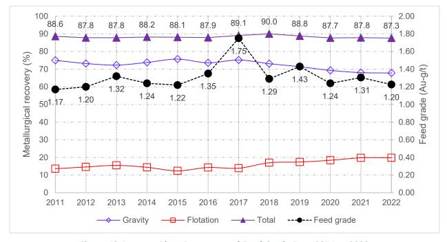
Figure 13-1: Plant Recovery and Feed Grade Data 2011 to 2022
