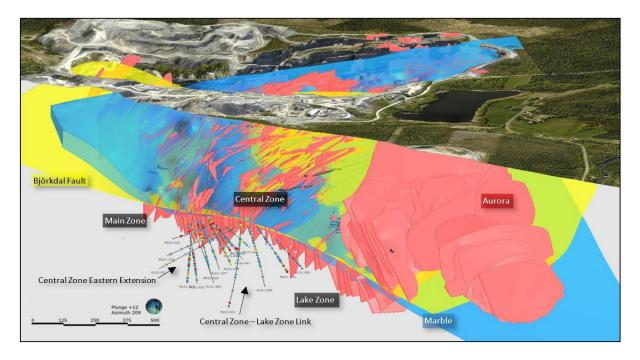
Figure 1: Perspective view of the Björkdal Mine looking towards the SSW highlighting the interaction of the veining (Red) Marble (Blue) and Björkdal fault (Yellow). Drilling of the latest Eastern Extension program is also shown.
