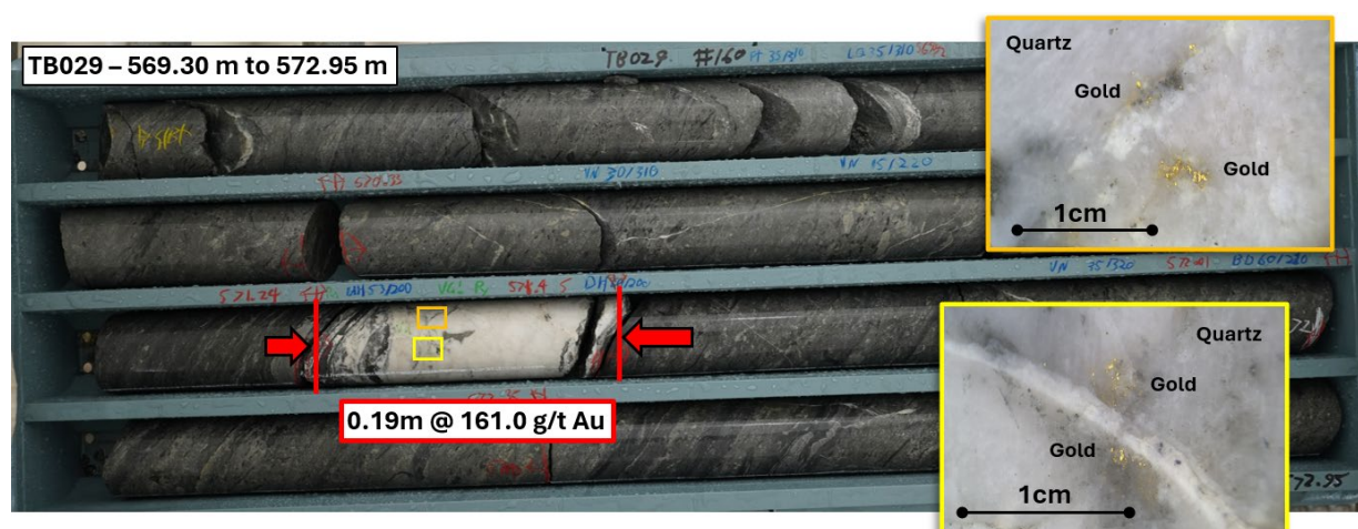
Figure 5. Photograph of True Blue intercept interpreted to be the Bearded Fault from TB029 - 161.0 g/t gold over 0.19 m (ETW 0.15 m) with inset showing close-up of visible gold within a quartz matrix at 571.25 m down hole.
