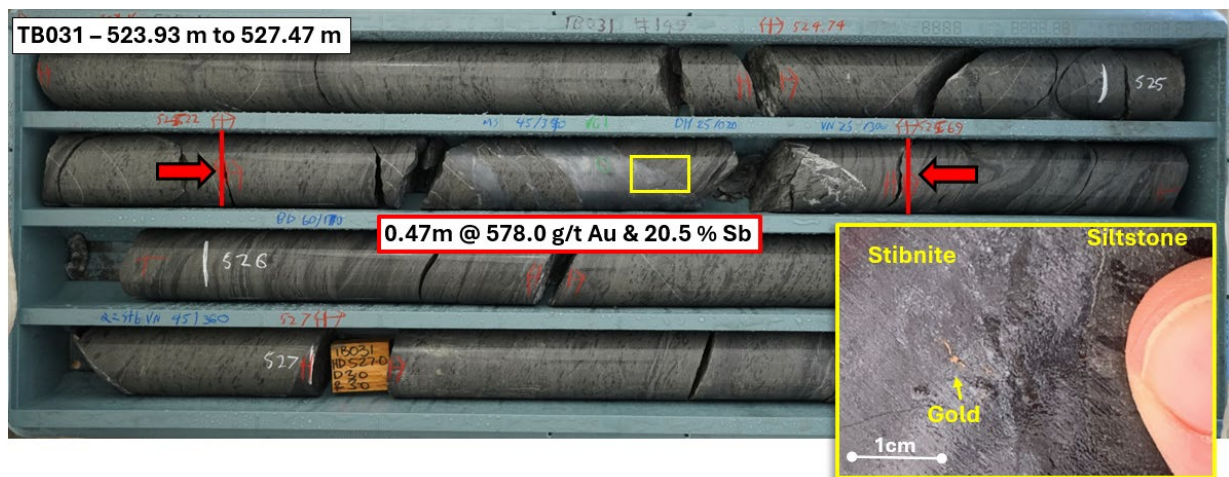
Figure 6. Photograph of True Blue intercept from TB031 – 578.0 g/t gold over 0.47 m (ETW 0.33 m) with inset showing close-up of visible gold within a stibnite matrix at 525.50 m down hole.
